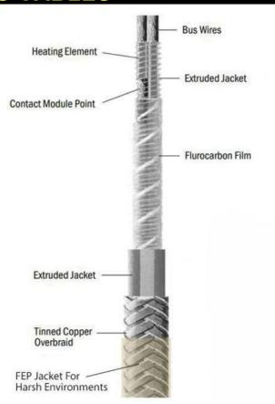
Our general purpose, constant wattage heating cable is a proven, reliable solution for industrial process temperature maintenance and freeze protection. A parallel heating core produces uniform thermal output over its entire length. Using a single power point, you can easily configure and install a heat tracing system as short as several feet or as long as 780 feet right in the field.
